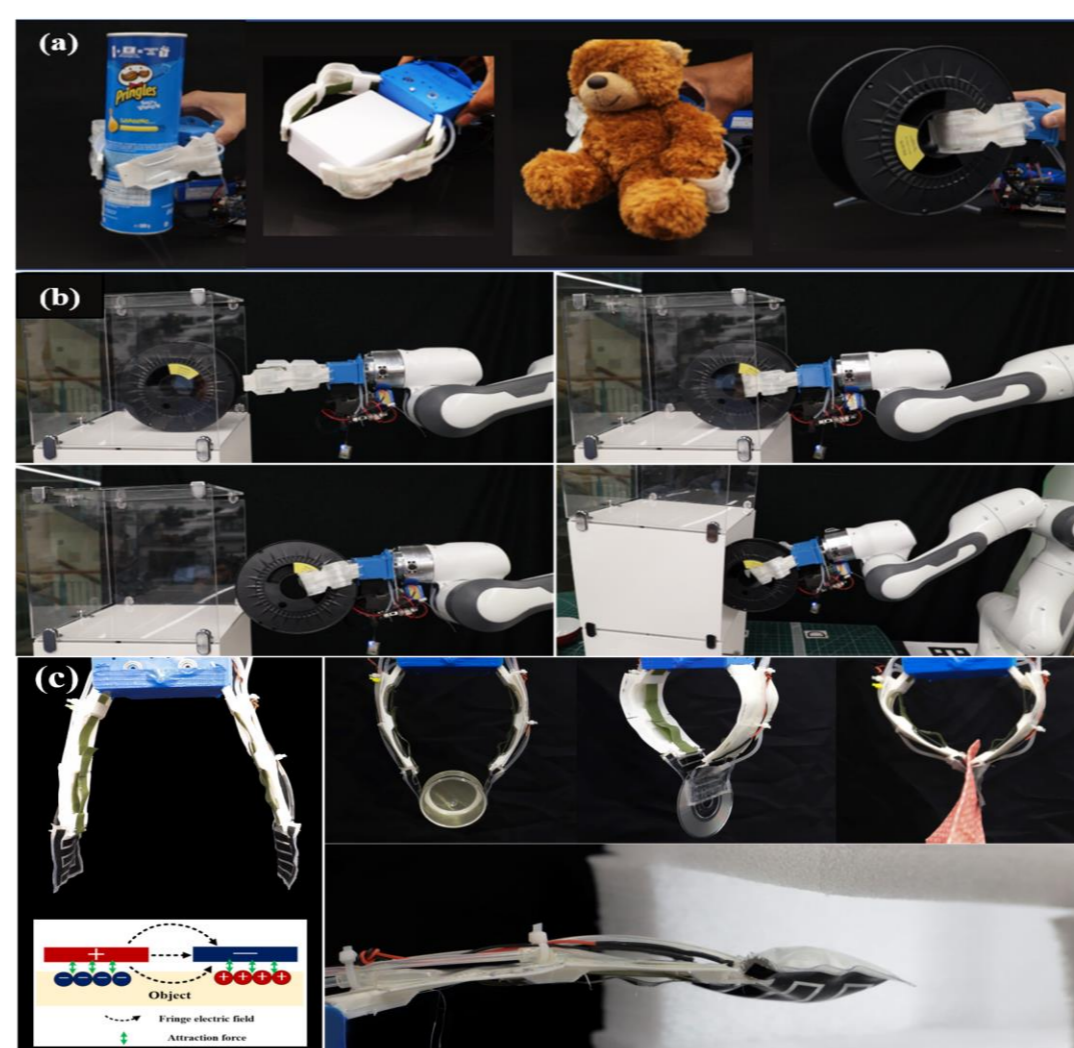
Fig. 3 (a) Grasping different objects (b) Implementing pick and place task (c) Grasping items with EA pads, and the pouch actuator helps to keep the EA pad in a firm shape
